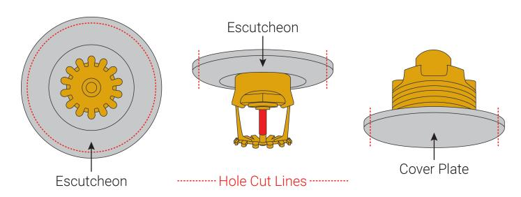
An appropriately-sized hole saw can be used to cut clean, smooth, and neat sprinkler pass-through holes in both your refacing ceiling tiles and mineral fiber backing panels. When cutting the holes in your Ceilume tiles, we suggest running the saw in reverse in order to keep the material from binding as the hole is cut.
